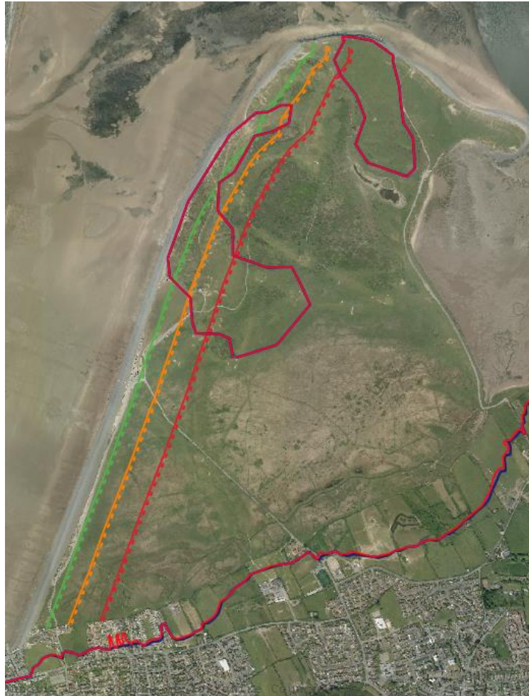
Figure 2-5. Aerial image of Westward Ho! showing the predicted barrier rollback positions for three epochs; short term (green line); medium term (orange line); long term (red line). The buffer lines for each epoch are demoted by the dashed lines. Flood extent 'dry islands' are also plotted over Northam Burrows.
