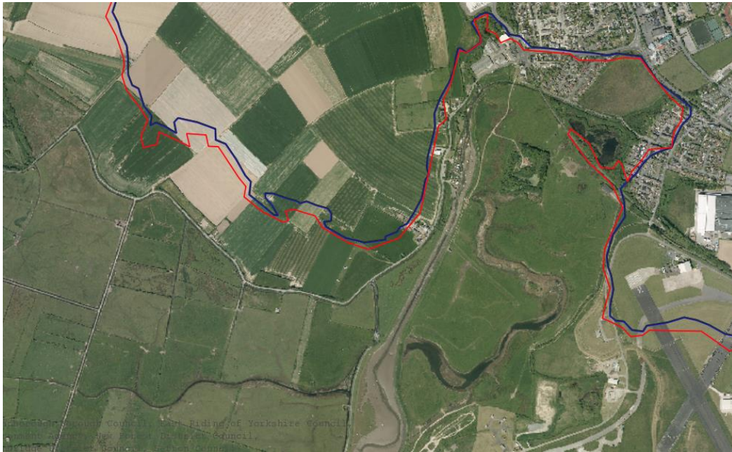
Figure 2-3. Aerial image showing Velator and parts of RMB Chivenor with the CCMA extent overlaid. Red line is the projected 1:200 yr line and the blue line is the projected position including the vertical and horizontal buffer.
