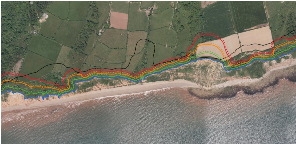
Figure 2-7. Aerial image showing the current cliff top position (blue line) and the predicted cliff position for the three epochs; short (green), medium (orange) and long term (red). The dashed lines indicate the associated buffer lines. The black line indicate the long term SMP prediction.
