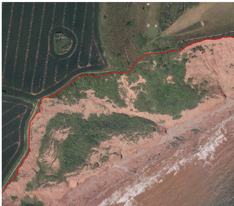
Figure 2-2. Example coastline section with manually digitised cliff line (red). The line is defined through a combination of vegetation boundaries and change in slope from LiDAR elevations.
