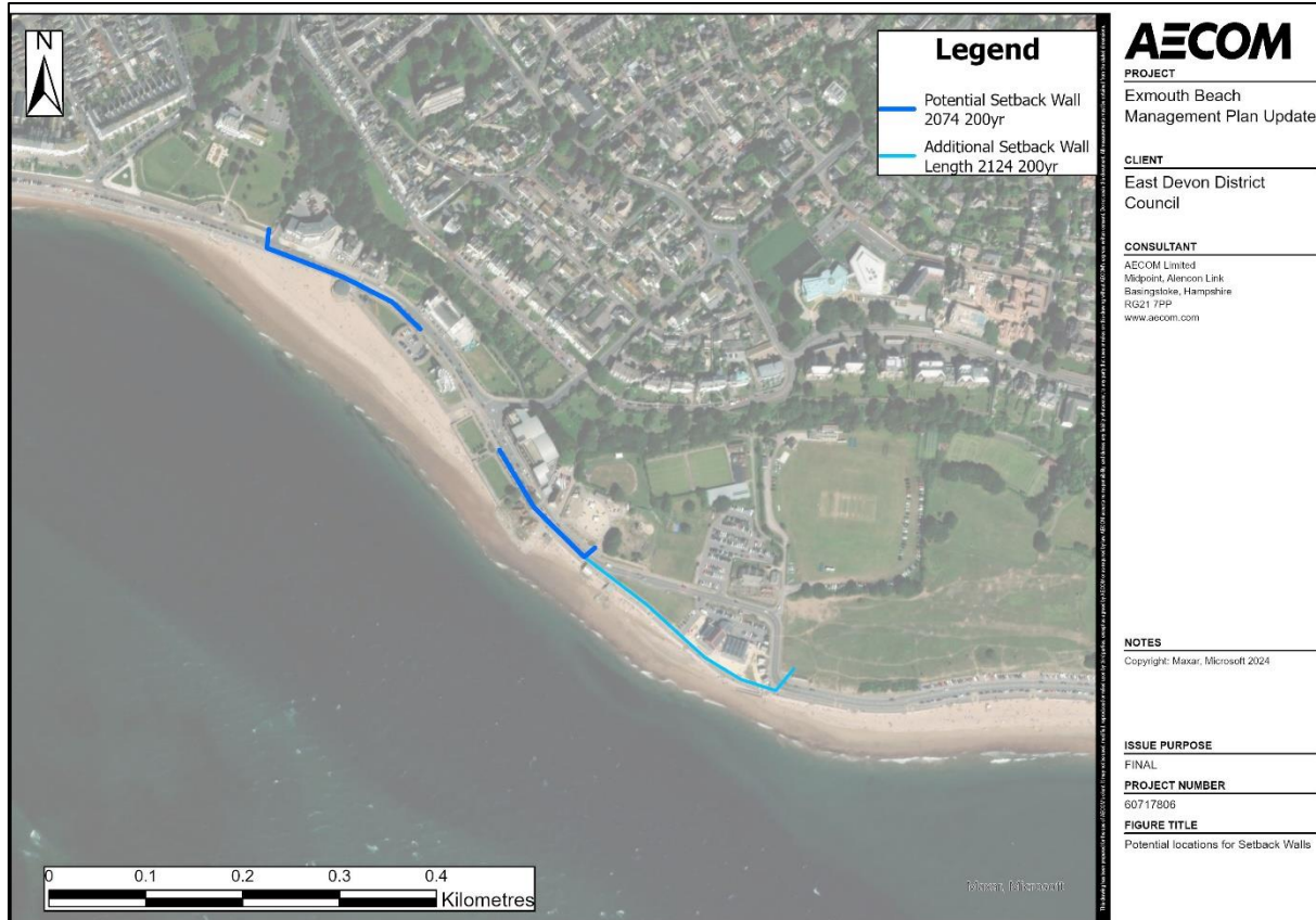
Figure 3-8: Setback Floodwall Alignment (as used in costing)
