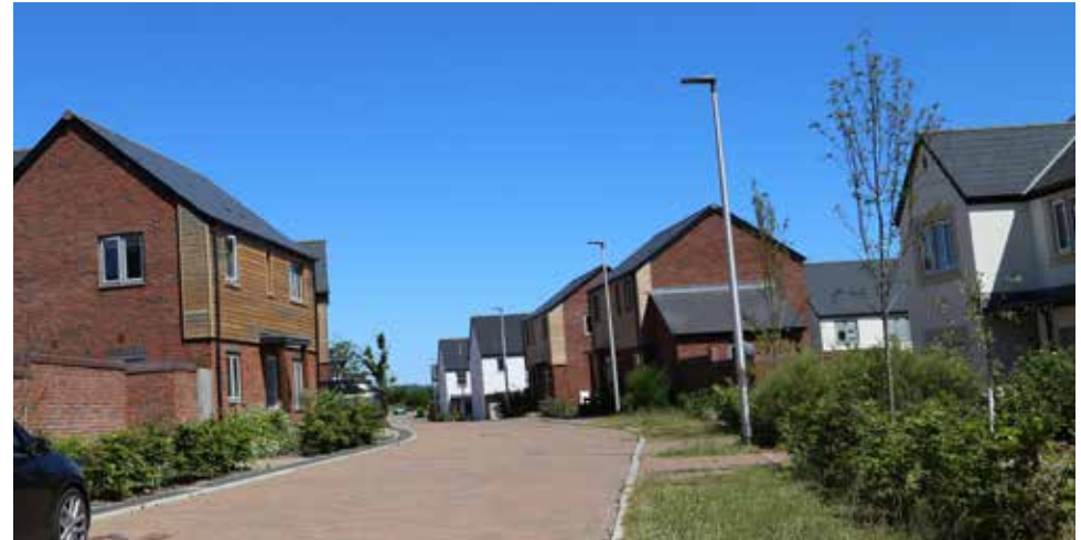
Figure 44: Good example of new developments and mix of materials including red brick, render and slate. Weather boarding adds a different texture but arguably is not a local vernacular material. Perhaps hanging tiles instead.
