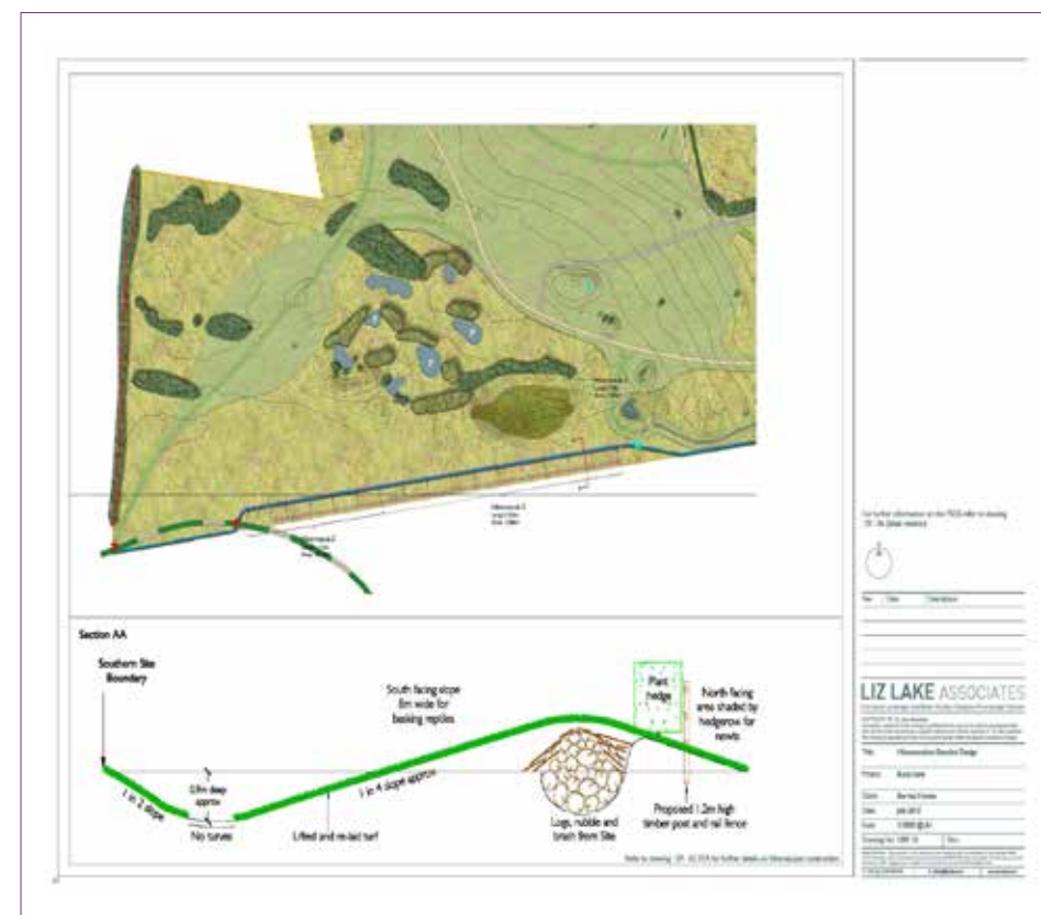
Schematic layout and design for the hibernacula at Maple and Stanford Park
