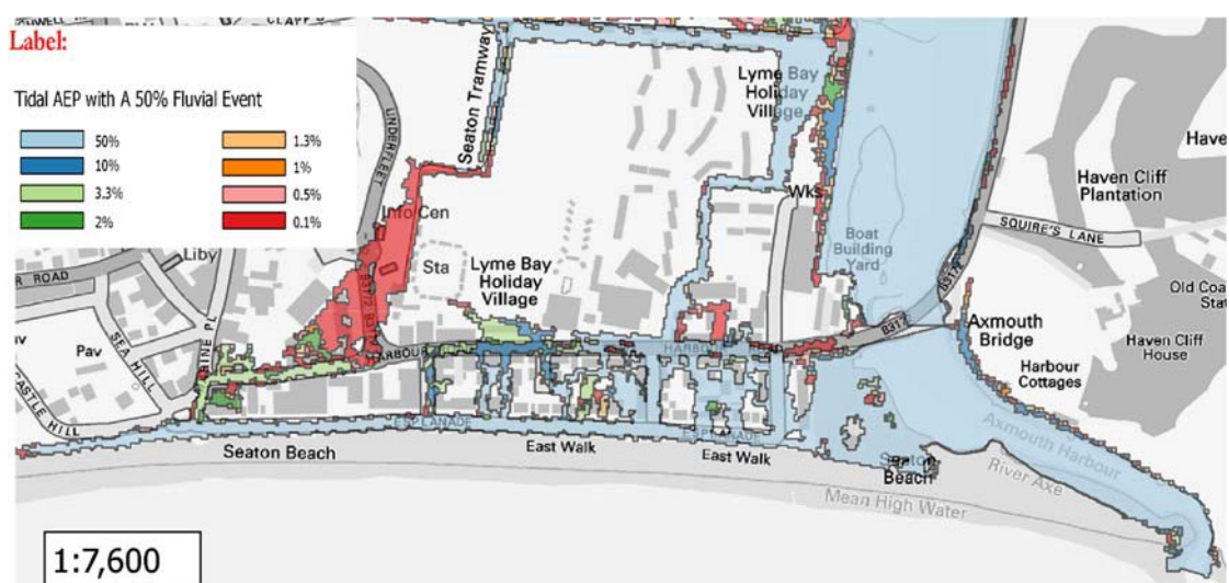
Figure 3.12 Present Day Flood Risk from Wave Overtopping of Coastal Defences Under a range of Return Periods
