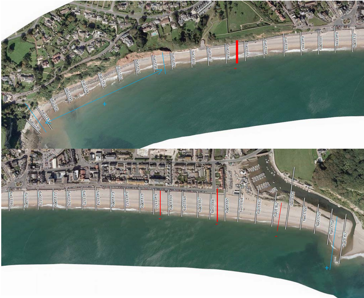
Figure 2-8 Map showing location of beach profiles with positive cross-sectional change shown in blue and negative cross-sectional change in red
