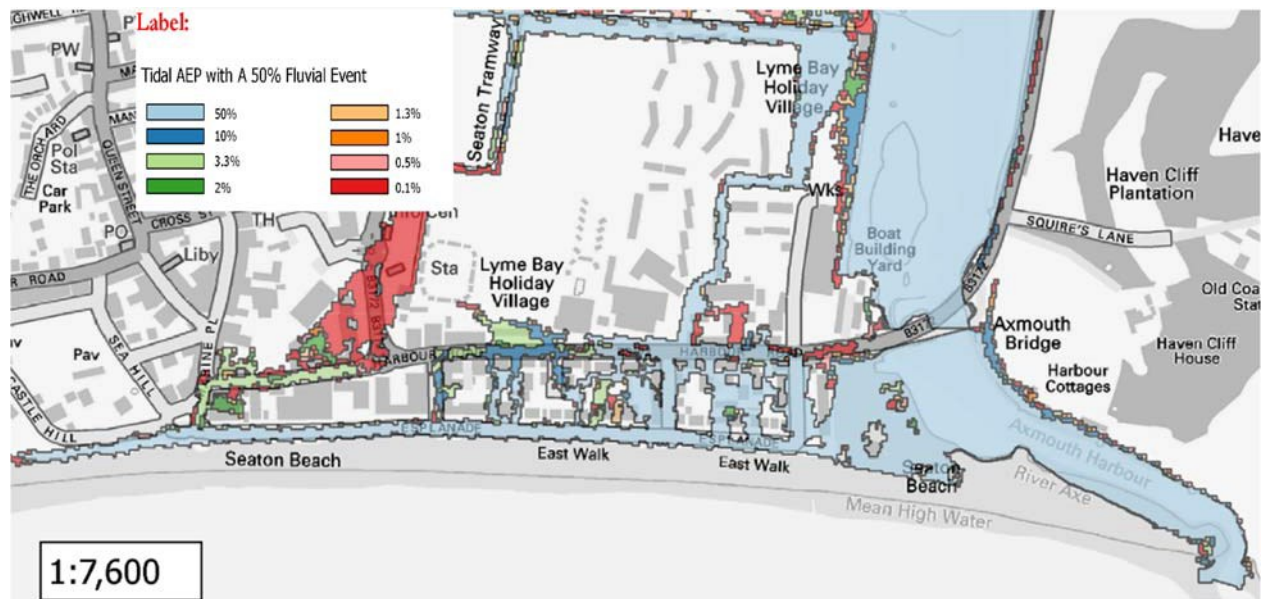
Figure 1-4 Present Day Flood Risk from Wave Overtopping of Coastal Defences Under a range of Return Periods Source: CH2M, 2017a
