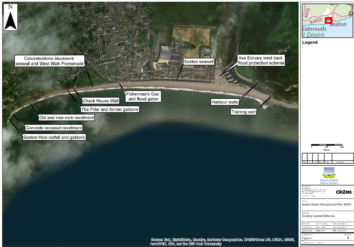
Figure 1-2 Existing coastal defences along the Seaton BMP frontage
