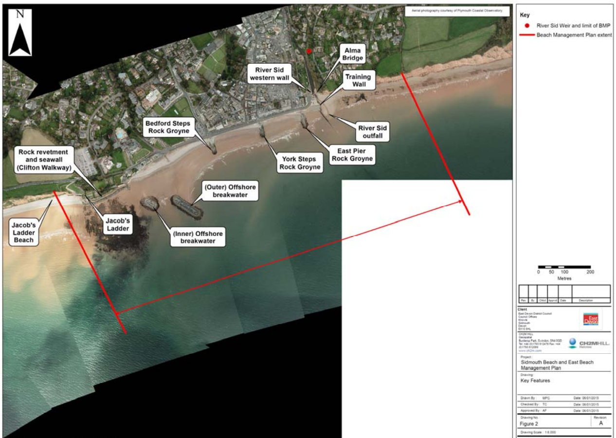
Figure 2-2 Key features along the BMP frontage
