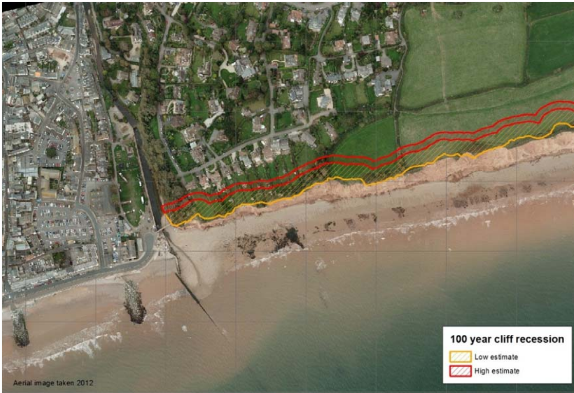
Figure 3-1 Cliff recession projection for 100 years at East Cliff (CUB7). Note the projection is made from the 2015 cliff top, but are overlain on the 2012 image for presentation purposes.
