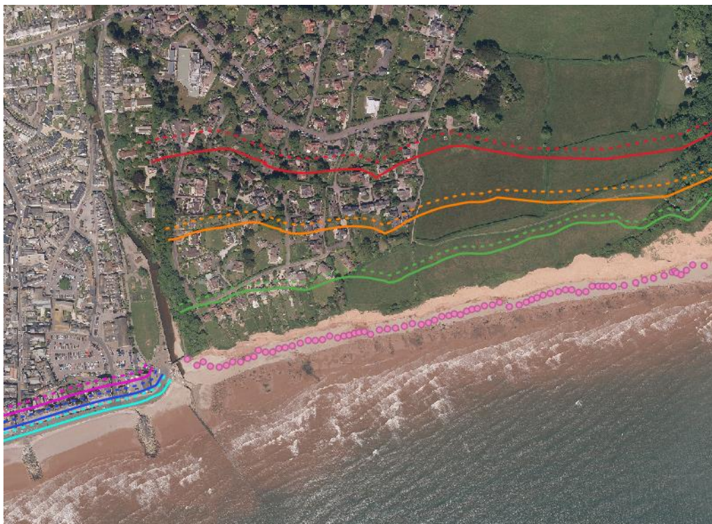
Figure 6-1. Snapshot of CCMA lines for Sidmouth (see Appendix A for full regional maps and legends). Pink dots indicate the location of profiles used to calculate historic retreat rates.
